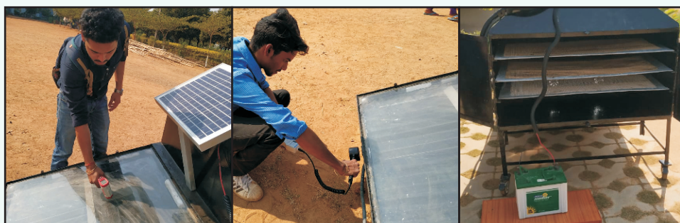
Plate-1: Experimental set up of Hybrid type of Solar dryer and testing of dryer
